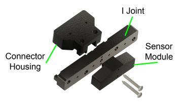
Reattach the Sensor Module to the I Joint using the two #8x1.25" Screws. Be sure to pull the wiring through the hole in the I connector as you press the sensor module into place, so that there is plenty of slack on the other side for the connector housing.
