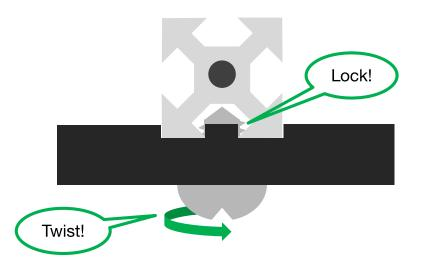
Every connection will be made with at least two screws. To ensure a tight fit, always tighten the screw furthest from the corner first, this will pull the extrusion into the corner. Once the outer screws are tightened, the extrusion will be fixed in place and the inner screws can be tightened.
