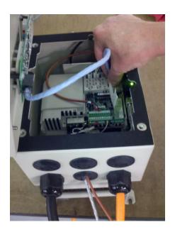
On the front face (face plate) of the VFD remove the soft rubber covers that hide the (4) screws. Remove the screws. Carefully open the face plate and disconnect the face plate's data cable from the main body of the VFD and set the face plate aside.
