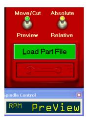
Start the ShopBot control software then go to Tools, Spindle RPM Control [TR].
