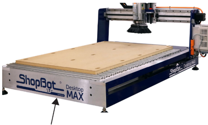
Front Lifting Points (along bottom of tool)
