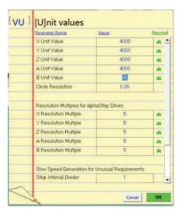
Open the control software and click Values > Display Values on the top menu bar. A yellow fill-in sheet will appear, as shown below. Change Display units B axis to degrees, and change Number of Axes to 5. Then click OK at the bottom of this sheet to save changes.
