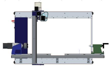
The headstock and tailstock have been shipped with their respective mounting hardware fastened to them. The headstock is mounted to a T-slot Plate with pair of T-nuts and flange bolts. The Tailstock is mounted with a pair of T-bolts with washers and nuts.
