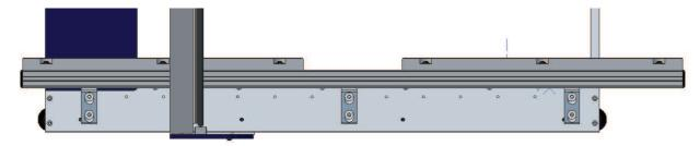
With the gussets aligned and square to the extrusion, slide the extrusion assembly forward such that the two holes in each gusset are aligned with their respective two holes on the MAX frame.
