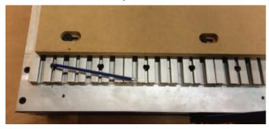
Use an M4 hex wrench to remove the spoil-board and aluminum decking and from the Desktop MAX.
