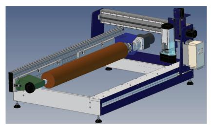
If turning parts less than 4.5" in diameter, the indexer can be alternatively mounted directly to the aluminum T-slot extrusion deck, where the limiting factor will be distance from the axial center of the indexer to the deck (2.25"). An extra set of 6x screws (002033) and T-nuts (002498) are provided for mounting in this configuration.
