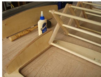
A rubber mallet may be needed to push the assembly together. Also check for excess glue that has pushed out.
