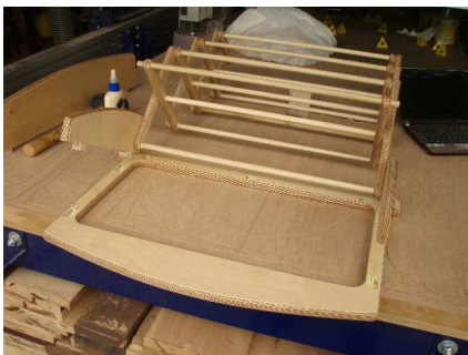
Then push the tenons on the side pieces into the mortises on the back piece.
