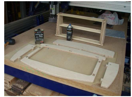
Before assembling the back half of the project rub all the parts with several thin coats of Min-wax WipeOn polyurethane. The folding dowl fixture can be opened and closed and sprayed with polyurethane.
