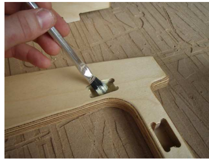
Fill the bottom of the mortise slots with glue. A small brush is useful to spread the glue on all edges of this joint to ensure a proper glue joint.
