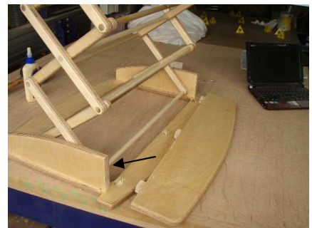
Attach the top in the same fashion as the side pieces by gluing the mortise and tenon joints together. Also add some glue to the top edge of the sides.
