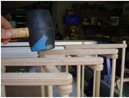
Pushing the dowels flush with the slats with a rubber mallet.
