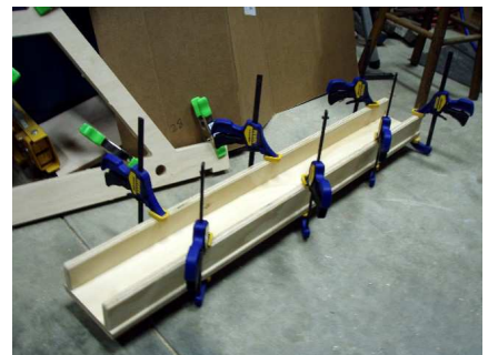
Glue the joints and clamp until the glue has had a chance to set up.
