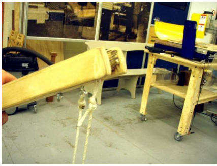
Eye hooks are mounted by eye just in from the end of the arm. One end of the string needs to be affixed as shown above.
