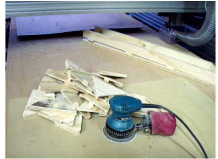
As the parts are drying sand all of the gusset pieces. These are the pieces with the giant pockets on the back side.
