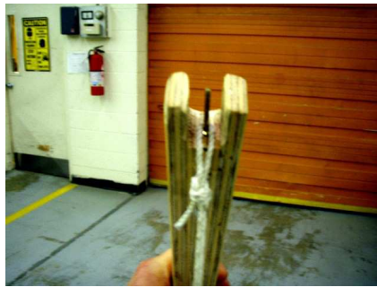
A center hook is mounted in the center of the arm. This string will let loose during launch.
