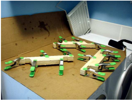
Clamp the assemblies for at least an hour so the glue can set up.
