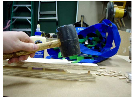
Using a rubber mallet lightly tap the two halves together.
