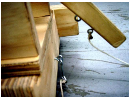
Notice the eye hook closest to the end of the arm is the one with the string tied to it. The second one back is left open so the firing mechanism can be hold to this.
