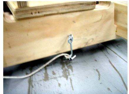
A simple screen door hook will work to hold the arm into the cocked position until it is ready to be launched.
