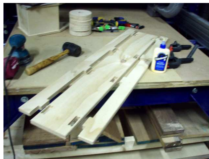
The bottom trough consists of one bottom and two side runners.
