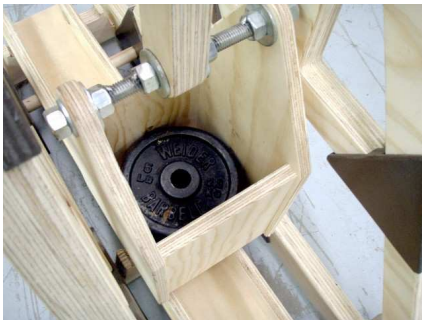
For this example, 20lbs is needed to launch a tennis ball. If you increase the projectile weight one must adjust the counterweight.
