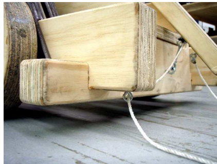
Eye hook placed along the bottom work as a track for constructing a trigger system.
