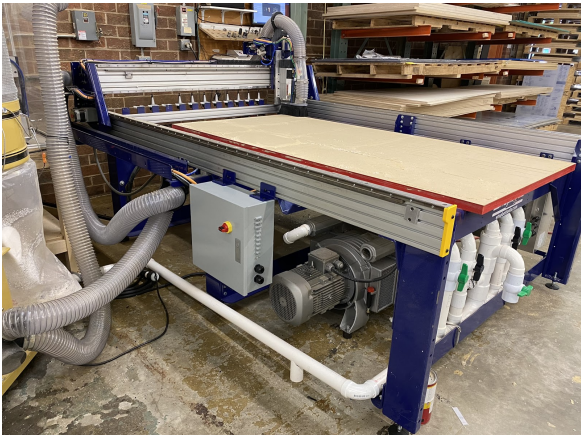
Figure 1: Standard Control Box mounted on 96x48 tool.
