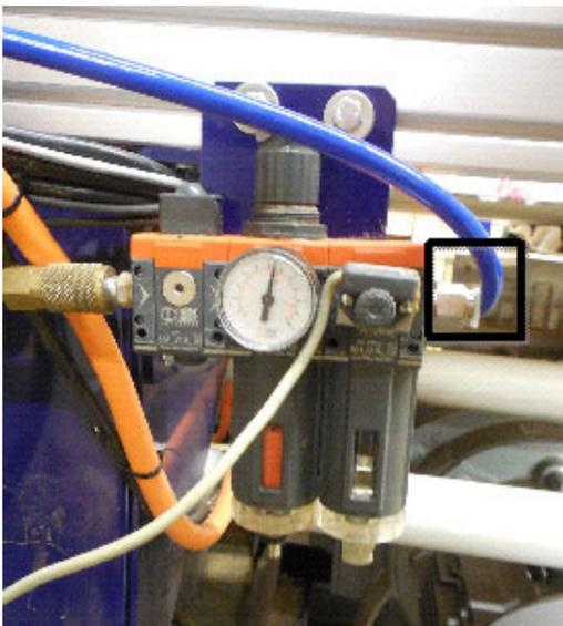
Insert one end of 3/8" tubing into the push-in fitting on the regulator side of the assembly.
