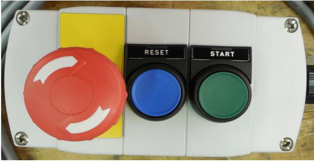
The ShopBot three button pendant allows the operator to locate the reset, start, and extra emergency stop buttons in a convenient location away from the control box. Control boxes may differ slightly from pictures shown, depending on which model is present.
