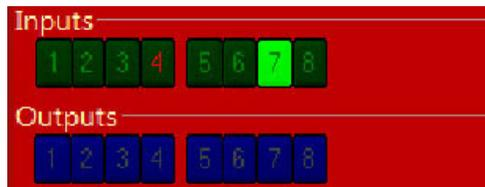
In keypad mode (K), move the Z-axis into the proximity target using "Page Up" on the keypad. The proximity switch will have a red LED lit until it comes across the proximity target, when it will turn off. Moving off the top of the target should cause the LED to come back on. This should also be evident in the ShopBot position screen when looking at input "5". Input "5" will appear green until the target is hit then the input goes black.
