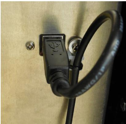
Plug in the provided USB cable into the control box connector, and make a loop in the cord for strain relief. Fasten the cord to the zip tie mount. Do not plug in the USB cable to the computer at this point, the software needs to be installed on the computer first.
