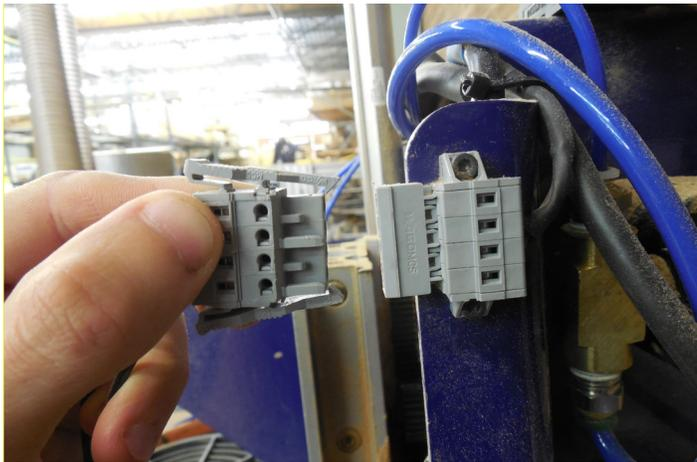
Insert plug end of the calibration and grounding clip into plug located near the wiring of the Z zero plate, on the YZ car. The calibration clip will be designated by the red grips and the grounding clip by the black grips.
