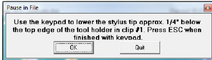
Note: This should only be a move in the Z-axis so that the tip of the drill rod is below the top edge of inverted clip. Do not move X or Y axes.
