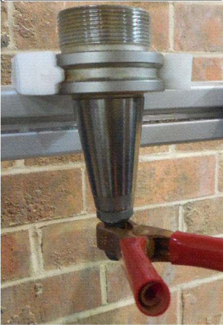
Place the red calibration clip on the bottom of the inverted tool holder in position #1.
