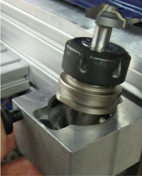
Press the button on the tool chuck to remove the tool holder from the tool chuck. Remove the tool holder from the tool chuck.
