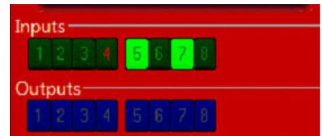
Release the button. The drawbar will close (captures tool holders). With the tool holder in place, input "7" will be lit and input "8" will go off.
