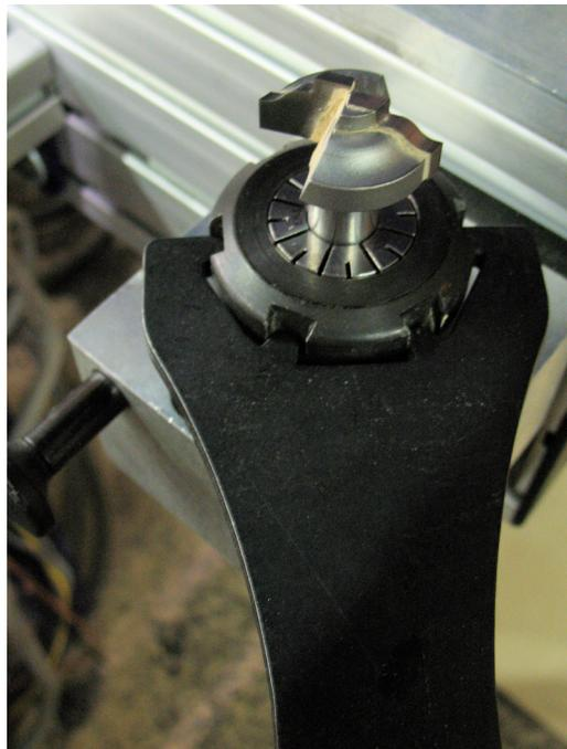
Tighten the collet nut to 100 ft/lbs with the ER32 spanner wrench. Do not over-tighten.
