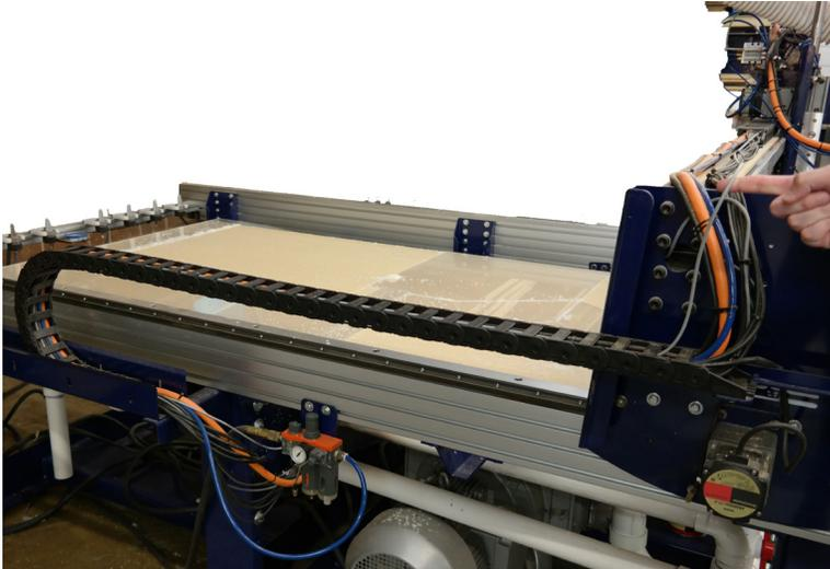
Route the gray cable from Wago connector through Y-Axis E-chain, through X-Axis E-chain, under table, through the Roxtec fixture on the side of the control box, and into the control box.
