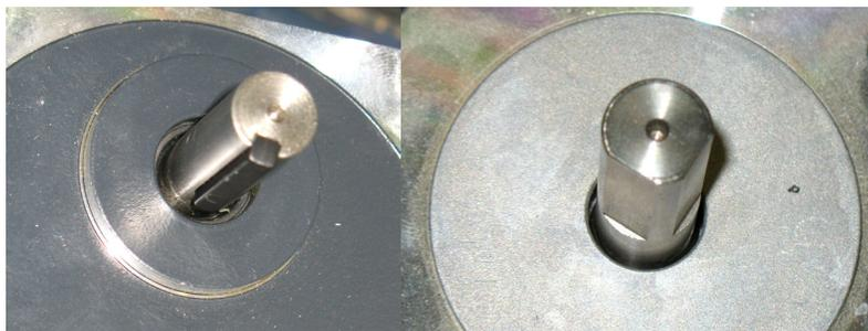
Depending on the model of motor, the motor shaft will either have a keyway or a flat to help keep the pinion from slipping on the shaft. If motor shaft is keyed, make sure that the key is still securely pressed into the keyway before putting the new pinion on. If the shaft has a flat, make sure that the set screw on the new pinion lines up with the flat.
