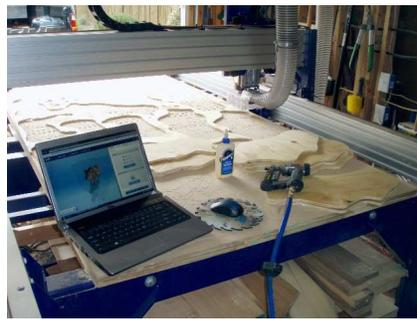
The Autodesk 123D make software labels each slice, so it is nice to keep a computer close by for assembly, this way the user knows which piece connects to each other.
