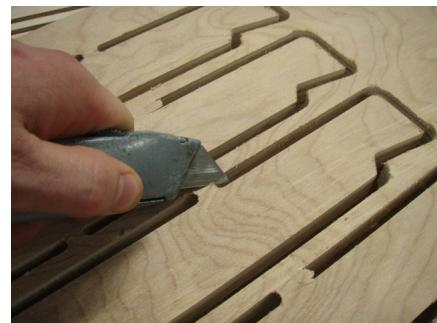
3. Tabs are used to hold all the pieces to the scrap wood attached to them. Use a utility knife to score these edges. Never try to push a piece out without cutting the tab; it will tear the grain on your project. Sand remaining tab flat.
