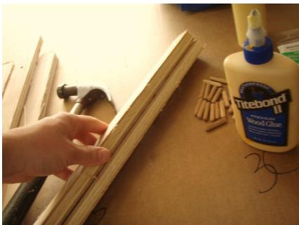
7. Push the pieces together so they line up. Make sure the ends are matched up and you haven't flipped the pieces around wrong.
