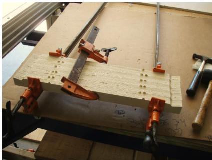
8. Glue, clamp and wait. If weight is going to be applied to this project at a later time one does not want to rush through these steps.
