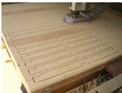
2. As the file starts cutting the profile of the parts, make sure the cut is going all the way through the work piece and into the table surface. If you need to adjust any part of the file make sure you do not remove the hold down or you will lose position.
