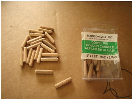
4. 1/4" x 1 1/4" dowels are needed for this project. Make sure the dowels are no longer than 1 1/4" or they will break through. One can sand them down or buy a shorter length.
