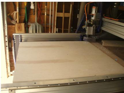
1. Included with the cut file is a hold down toolpath that shows where it is safe to put screws. Run this file separately from the cut file so you can screw down the work piece, or if you have a different size board or different type of hold down, disregard the file.
