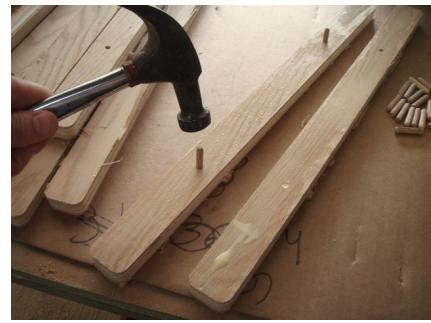
6. Lightly tap the dowel pins into place. They are here to help line things up.
