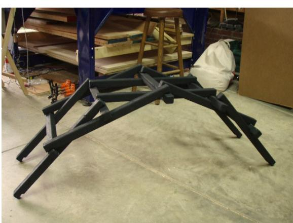
Note the above two pictures. By simply pulling one piece out of the bridge the entire thing collapsed.
