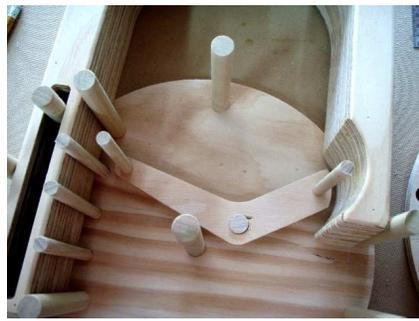
Install the lock over the 1/2" stub dowel and install a length of 3 1/4" dowel that is 5/16" dia. Into each end.
