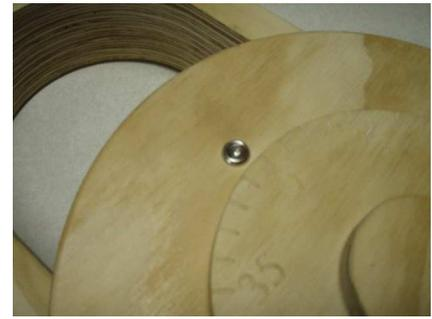
To help locate the front marker point, a decorative screw can be installed here. This is a good idea so the user has a reference point while twisting the knob.
