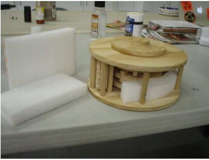
At first the wheels can stick to one another. Wedging in a piece of foam, rubber, etc. will apply just a little bit of tension on the center wheels.
