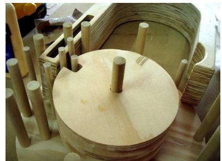
Finally repeat the first step and glue a piece of the rectangular stock into the third wheel, having the rectangular piece face down and be flush on top.
