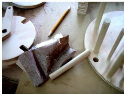
The remaining hole calls for a 5/16" dowel; however, it should be sanded down so that it fits through the "U" slots without any friction.
