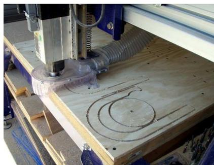
As the file starts cutting the profile of the parts make sure the cut is going all the way through the work piece and into the table surface. If you need to adjust any part of the file make sure you do not remove the hold down or you will lose position.
