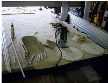
All of the exterior edges can be routed with an 1/8" round over. This will help keep the project each to handle and avoid any sharp edges.
