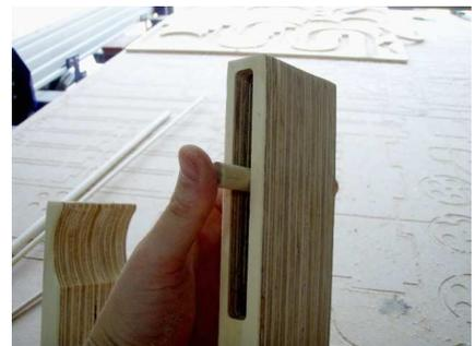
Test this dowel in the "U" fixture and keep sanding until it moves at ease and there is no friction.
