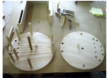
Install 10 pieces of dowel that are appx. 4" long. Also install the two lengths dowel that are 3/4" long, one into the back and one into the face.
