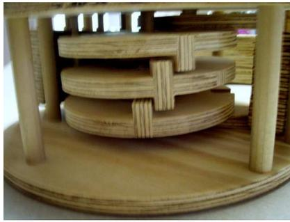
Twist the knob and make sure all three circles catch each other like above. This catching mechanism is what will be done and undone throughout the dialing of the combination.
