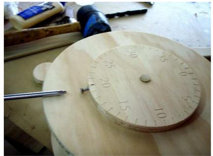
The first wheel needs to be permanently attached to the center dowel. Drill down into the first wheel and attach to the center 1/2" dowel with a screw and glue.
