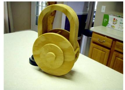
Simply push the "U" arm back down and rotate the dial, this will reset the lock and it will not open until the three proper numbers are reentered into the combination.
