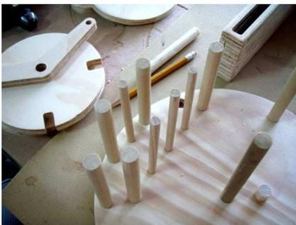
Four pieces of 5/16" dowel that are 4" long can be installed at this time.
