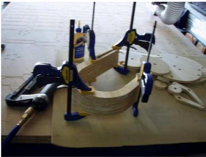
Once all of the "U" shaped parts are together apply clamps and allow the glue to dry for at least one hour.
