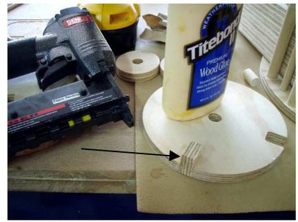
Using the long rectangular piece cut one section 1/4" longer than the depth of the plywood being used.
