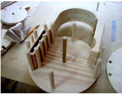
Drop in the "U" assembly with all of the dowels in place on the back side.
