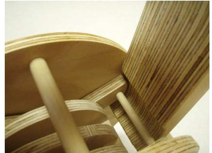
The lock arm will rotate down and allow the arm to come out of the base.
