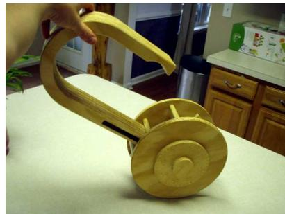
The upper portion will rotate on the dowel that holds it in place.
