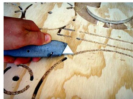
Tabs are used to hold all the pieces to the scrap wood attached to them. Use a utility knife to score these edges. Never try to push a piece out without cutting the tab, it will tear the grain on your project. Sand remaining tab flat.
