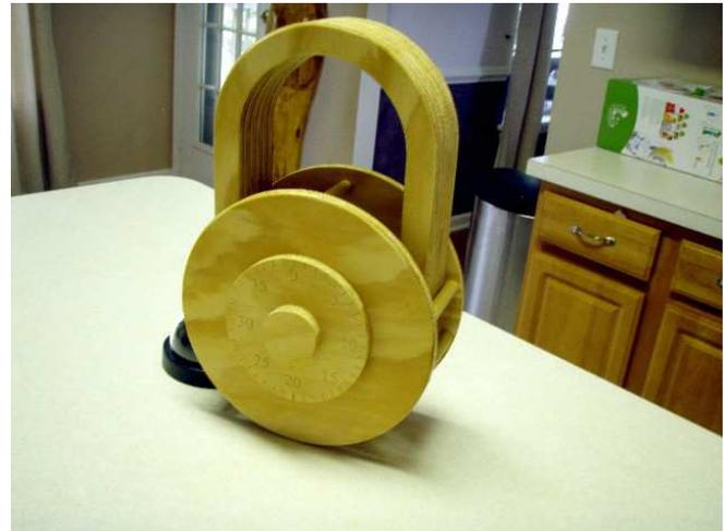
Remember each padlock will have a different combination. It all depends on how the user fastens the front dial and first inner circle to the center dowel. The lock has to be pretty dead on for the counter arm to open and the lock to open. However after a few times of testing your numbers you will know your exact combination that works every time.
