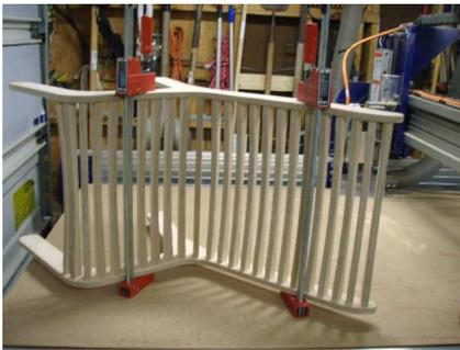
It can be useful to get a 3rd hand from an innocent bystander to help line up all of the slats into the pockets. Once this has been done clamp the project together and let the glue set up overnight.
