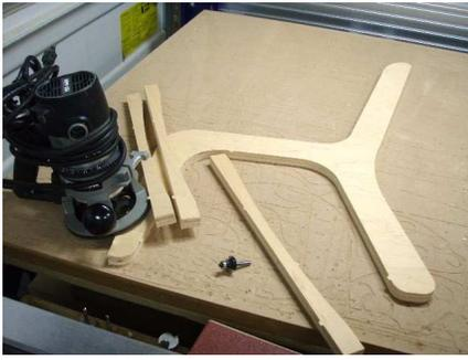
1/8" roundover is needed on all edges for this project to fit together. If one does not want their project routed, the mortises will need to be modified with a dog bone.
