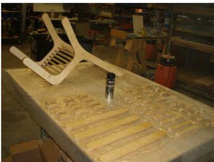
If space is available use Minwax WipeOn Polyurethane to wipe a finish on all the parts before assembly. If not, glue the chair up and spray the entire project with a spray polyurethane.
