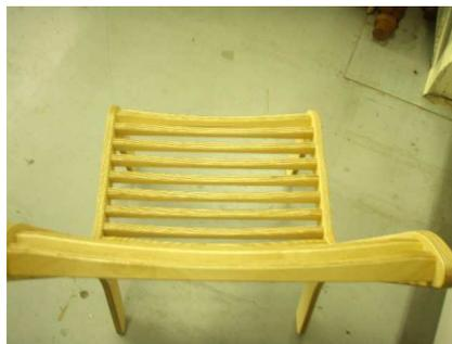
Once the finish has dried, rub the surfaces down lightly with a 220 grit or higher sandpaper to smooth the finish back out.
