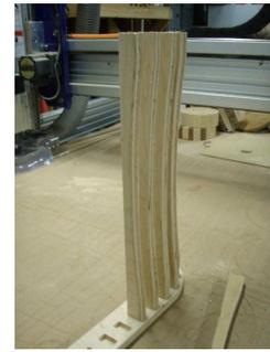
Apply glue in the pockets and work your way down from the top of the chair to the seat. Make sure all of the curved sides are pointed towards the front of the project.
