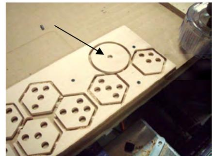
Note that all of the holes should be cut through the piece except for the hole on the base piece. This is only a pocket that goes half way through the wood.
