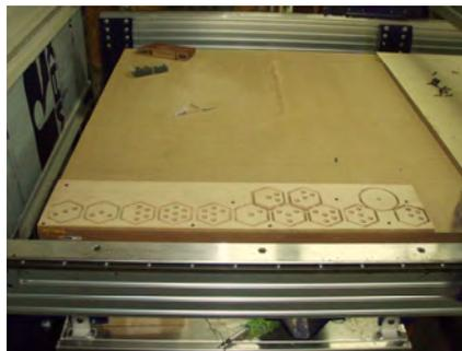
Before removing the work piece check to make sure the profile pass cut all the way through the material.
