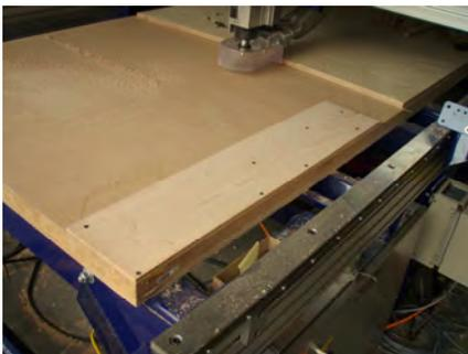
Depending on the machine you are cutting this file with, you will need to account for a hold down method. If using screws, simply reference the cutting area to a safe area to install the screws.
