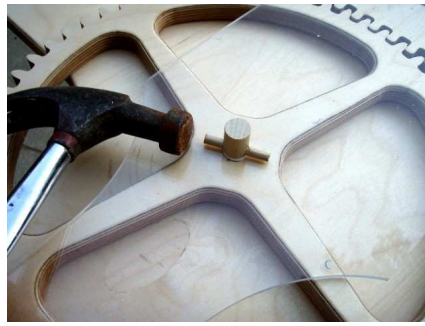
Measure, drill and insert some smaller dowels to help keep the plexi in place over the gears.
