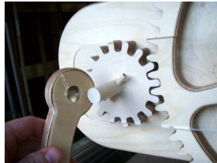
Apply some glue and insert the handle. Use glue on the end of the handle that is not a through hole. The through hole will be used as the physical handle that turns the gears.
