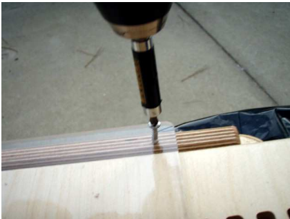
No more than a 1/2" in length screw is needed for these two holes.
