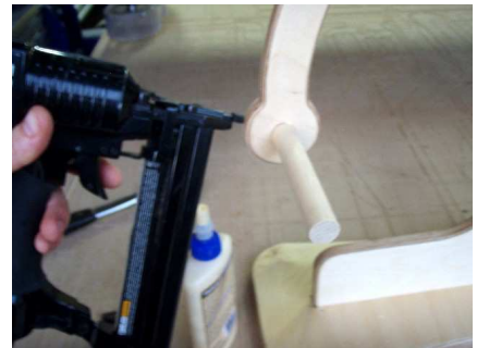
Glue in the dowel handle. Add a brad nail for extra strength.
