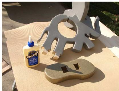
Make sure the tenons on the bottom of the elephants feet fit into the pockets on the base. Sand them if need be, just do not force and break off the tenons.
