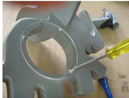
To ensure the Plexiglas is not cracked by over tightening, use a hand driven screwdriver and put the screws in by hand.
