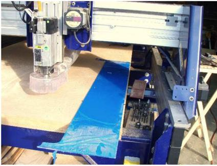
Plexiglas is cut at a much higher RPM and uses a O flute bit to cut. This bit is included in the Router Bit Starter Kit.
