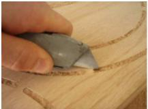
Tabs are use to hold all the pieces to the scrap wood attached to them. Use a utility knife to score these edges. Never try to push a piece out without cutting the tab, it will tear the grain on your project. Sand remaining tab flat.
