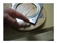
This file comes with 4 holes in the bottom piece that are spaces specifically for the lazy susan hardware used in this picture. The lazy susan purchased by you could have different hole layouts and the file could use some adjusting.
