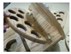
Insert glue into the pockets. Push the shelf into these pockets and allow to dry.
