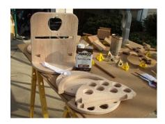
At this point stain all of the pieces to the desired color. Also apply polyurethane to the project after the stain has had time to setup and dry.
