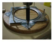
This bottom piece is ready to attach with four screws. Some small screws approximately 1/2" long will work fine.
