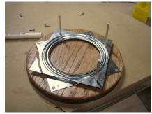
Use some scrap dowel pieces to line up the hardware with the bottom piece. The hardware will be attached to this piece first, the dowels will be removed and screws will go up through into the fixture.
