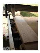
Included with the cut file is a hold down toolpath that shows where it is safe to put screws. Run this file separately from the cut file so you can screw down the work piece, or if you have a different size board or different type of hold down disregard the file.
