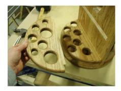
Note the size of the holes. The bottom shelf has smaller holes to help keep utensils standing straight up and down. However, make sure the upper shelves holes line up with the holes of the bottom shelf.
