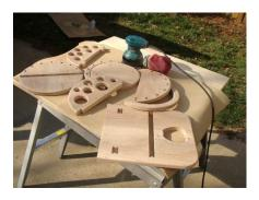
Sand all the parts evenly at this step. It is much easier to get to all of the parts at this state then before it is glued up. Putting a 1/4" roundover on all of the edges adds eye appeal to the project.
