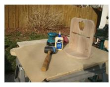
Glue the base to the center piece. A rubber mallet might be needed to push the center piece into the base piece.
