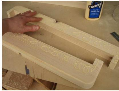
There are no fasteners used for assembling this project, so a proper glue joint is necessary to hold the pieces together. Spread glue evenly on both surfaces.
