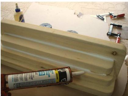
For this example the edges of the boards were routed with a 1/2" roundover. So a caulk line is being installed in the inside corners to be smoothed round to match the routed edge.
