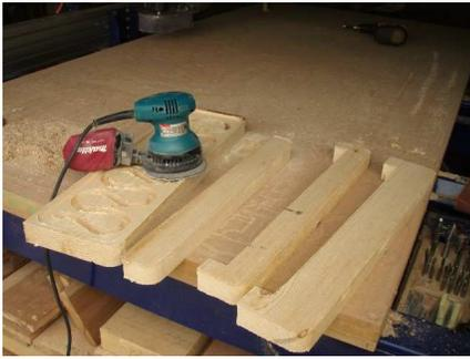
A random orbital sander should be used on all of the surfaces and hand sand paper to knock down the sharp corners. One can also add routed edges if desired.
