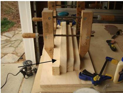
Clamp the back pieces together and let them setup before gluing to the top piece. Note the extra board used just for clamping purposes due to the cutout on the back of the back piece.
