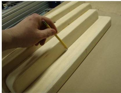
Flush the back pieces with the back edge of the shelf. A scribed line will help show where to place the glue.
