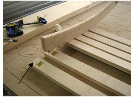
Move over to the seat portion of the chair. Fill all of the mortise pockets and start pushing the chair pieces together. Note the distance of the pockets from the end of the slats. The ones with the longest distance are used on the seat portion.
