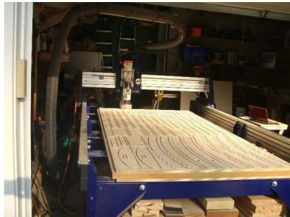
Two chairs can easily be cut from a 4' x 8' piece of plywood. Simply increase the quantities in the file and re-toolpath.
