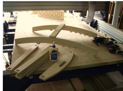
After the back slat has had time to setup, flip the assembly over and prepare to glue up the remaining parts of the chair.
