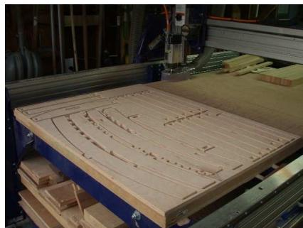
As the file starts cutting the profile of the parts make sure the cut is going all the way through the work piece and into the table surface. If you need to adjust any part of the file make sure you do not remove the hold down or you will lose position.
