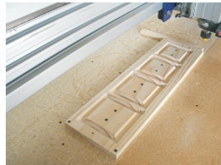
After flipping the material width-wise, run the SideB file and label the four 'B' parts after machining
