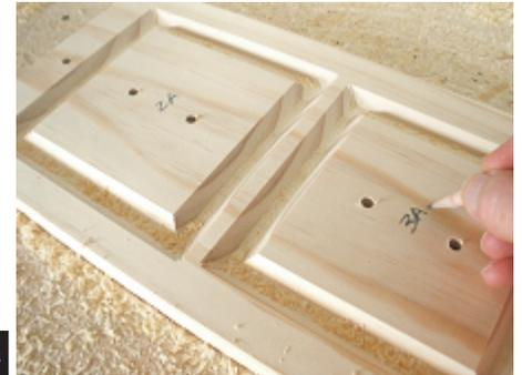
After machining and labeling the **SIDE A** file, flip the board over across the (shortest) width. Insert two alignment dowel pins into the holes in the spoilboard and replace the board onto the pins with the plain side up. Re-apply a secure hold-down method.
