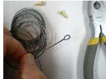
**fig. 5a** Twist/Loop Wire
