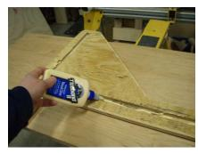
When assembling this project consider the fact that weight will be applied constantly when this project is put to use. So take your time and glue, screw and nail it properly.
