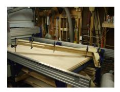
After gluing make sure the project is clamped together and the clamps are left on until the glue has had time to setup.
