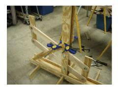
Start assembling the arm. Note the middle holes are not centered, they are off to one side, they need to be positioned as pictured above.
