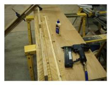
A nail gun is also a great way to temporarily hold the parts in place before clamps can be installed.
