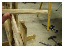
One of the small squares has a pocket on the bottom side, glue and screw this to the support that is below the upper arm.
