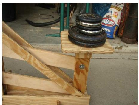
No weights laying around? No problem. Set a 5 gallon bucket of water on the pedestal, start filling it up, when the column crushes, have them weigh the bucket of water on a scale and convert water gallons into weight.
