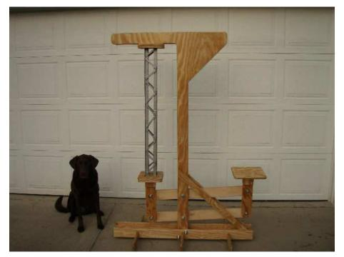
Start applying waits until the tower has crumbled apart.
