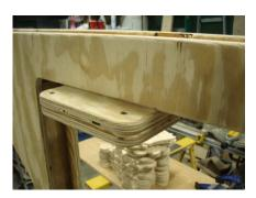
Glue and screw to make sure this project holds together once the weight is applied.
