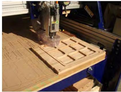
Secure the game board piece to the table surface, for this example screws are put in each corner at a safe distance from the cutting area.
