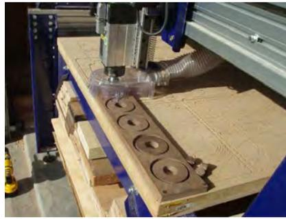
Do the same thing for hold down as done on the X's. Note the center of the O's can come loose and pop out during the cut. Depending on the grain of the wood a bigger tabe may be needed to keep these centers from popping out.
