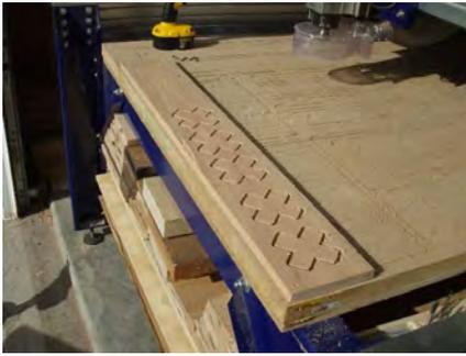
A scrap piece of red oak is used for the X's. Simply locate safe locations for the hold down screws and install one in every corner.
