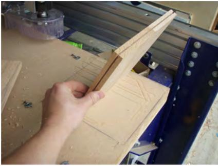
Remove the screws from the hold down. Grab the piece of wood and flip it over in the X position. Note that the edge of the board that was at X=0" will now be at X=10".
