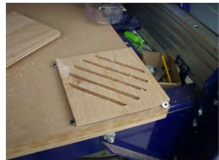
This is what the project will look like after the first toolpath. At this point take a pencil and trace the perimeter of board. Next you will be flipping the board over and it is very crucial that it is lined up with the first toolpath.
