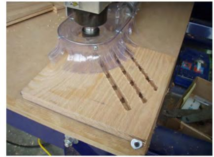
Reinstall the hold down, load the second cutting file which also includes the profile cut that removes the project from the scrap. During this cut the previous toolpath will be exposed from the underside.
