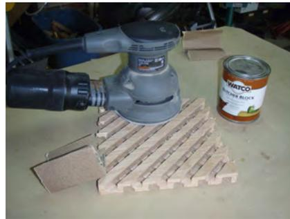
Thoroughly sand the projects surfaces with a power sander. Also use hand sand paper to knock down any sharp corners. Follow any manufacturers finishing instructions or simply rub food grade mineral oil into the wood until it coats evenly.
