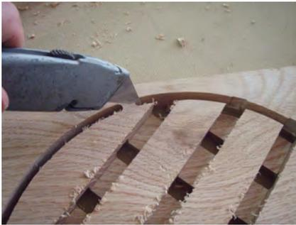
Tabs are used to hold the project to the waste material. This keep the parts from slipping during the cutting process. Simply find these tabs, score them with a utility knife, remove the project from the waste material and sand off the tabs.
