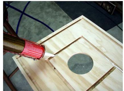
Start by laying a line of adhesive on all of the inside grooves.
