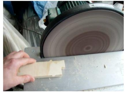
Sanding off the tabs with a disc sander speed up the process of finishing this project.
