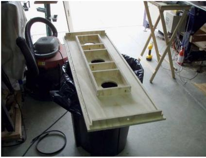
Following the same order of operations add the other pieces by applying adhesive to all of the grooves and then installing the shorter pieces to the ends.
