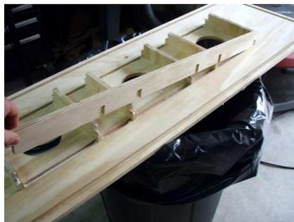
Add the two longer inside pieces and make sure they are pushed down into the grooves.
