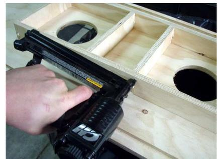
A pin nailer will help hold all of the pieces into place until the adhesive has had time to setup.
