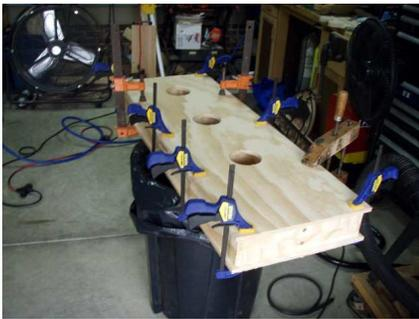
Flip the pieces onto each other and apply clamps. The two halves will now glue up and match each other perfectly.
