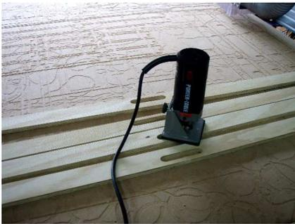
A round over edge that is routed on all of the outside edges will make this project more comfortable for carrying and add eye appeal to the overall project.
