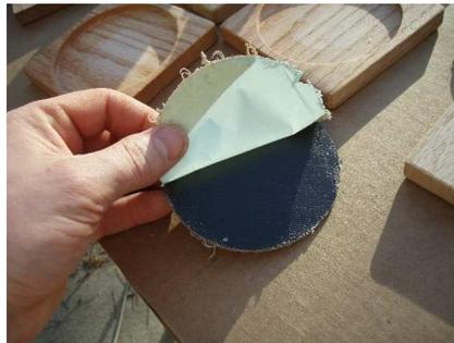
Once the backer is peeled off from the tile one will need to stick it to the wood within a few seconds. If you did not use a self adhesive tile try gluing the tile to the wood.
