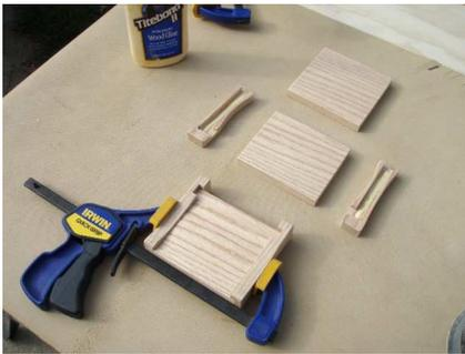
Quick grip clamps work great for applying pressure to this project. Put one on each of the side/cap glueups.
