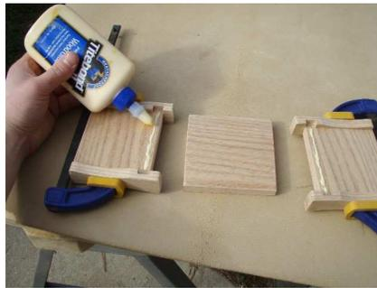
Apply a small amount of glue along the bottom of each side piece. Also put some glue on two of the edges of the bottom piece that fits into this groove.
