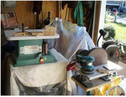
This project has straight, inside and outside edges. A good combination of hand, orbital, spindle and disk sanding will whip this material into smooth shape.
