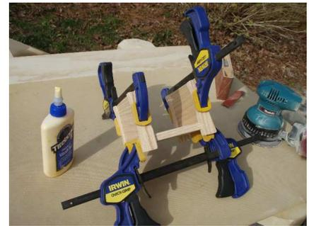
Two more quick grip clamps will hold the whole project together. Have a square close by to ensure you have glued the sides at 90 degrees. Allow several hours for the glue to setup before removing the clamps.
