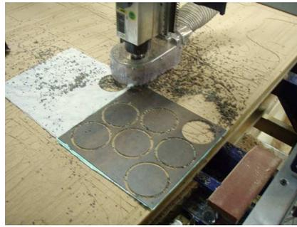
There is a provided toolpath to cut the circles from these 12" x 12" tiles. No tabs are used because of the carpet tape. Also note in the file the bit that is used and the speed rate to cut these.
