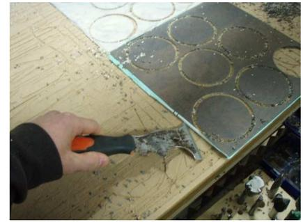
Depending on the tile one chooses, different feeds and speeds and bits will be used. Feel free to experiment. When the circles are cut pry them off keeping the backer on the tile.
