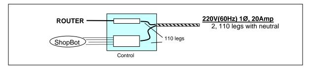
2 pole, 30A circuit. The 2 legs will be split into two 110V circuits inside the Control Box: one to the control circuits, and one for the router. Refer to drawing listed below, included in the Control Box, for detailed wiring information.
