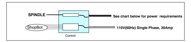
110V single phase, 20A circuit for the Control Box plus the circuit for the HF spindles (see pg 4 for spindle power specifications). Refer to drawing listed below, included in the Control Box, for detailed wiring information.
