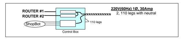
220V 2 pole, 30A circuit. The 2 legs will be split into two 110V circuits inside the Control Box: one for the control circuits, and one for the two routers. Refer to drawing listed below, included in the Control Box, for detailed wiring information.
