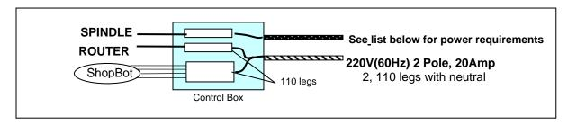
220V 2 pole, 20A circuit, one leg for the Control Box and for the Router, plus a 230V 3-phase circuit for the HF spindle (see pg 4 for spindle power specifications). Refer to drawing listed below, included in the Control Box, for detailed wiring information.
