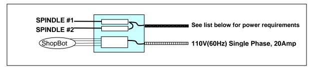
110V single phase, 20A circuit for the Control Box plus the circuit for the HF spindles (see pg 4 for spindle power specifications). Refer to drawing listed below, included in the Control Box, for detailed wiring information.
